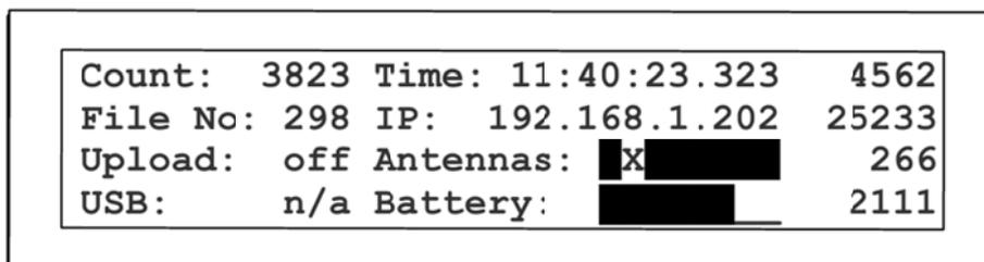
The left-to-right order of the antenna indicators mirrors the left-to-right order of the ports on the back (or right-to-left when looking from the rear).
