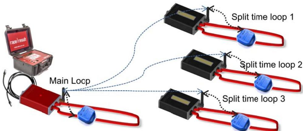
Note that the LoopBox has an internal buffer for 1000 detections. Even if the connection between LoopBox and Active Extension is interrupted, the detections will not be lost: once the connection recovered, the LoopBox will transmit the buffered detections. Thanks to the precise internal clock of the LoopBox, the detection time will still be correct and precise.
